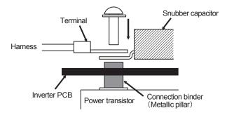
Procedure on tightening harness (snubber capacitor) and power transistor with screw. A metallic connection binder is set in each hole of the inverter PCB of "P", "N", "U", "V", and "W" beforehand. Then tighten the harness (snubber capacitor) and the power transistor with the screw together. (Set the harness wires to be fixed to "U" and "W" with screws in respective holes after passing them through IC21 and 22.) (Connect snubber capacitor with "P" and "N".)
