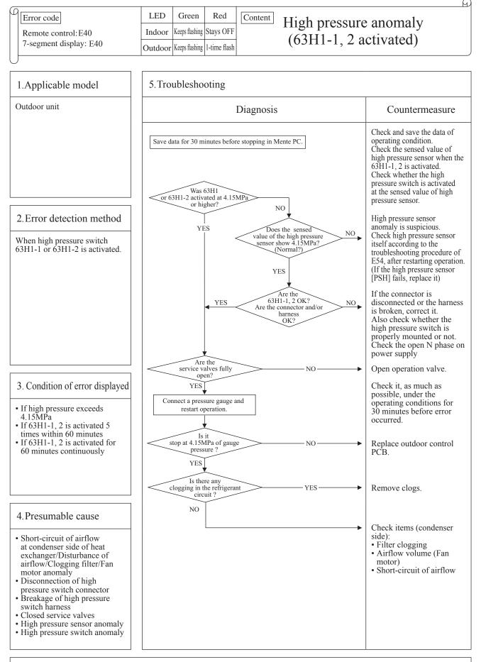
Note: If the error does not recur, connect the Maintenance PC and continue to collect data.
