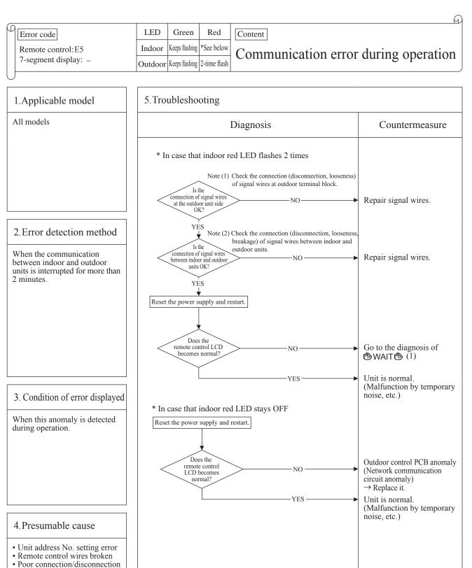
Note: When the pump down switch is turned on, communication between indoor and outdoor units is cancelled so that "Communication error E5" will be displayed on the remote control and indoor control PCB, but this is normal.
