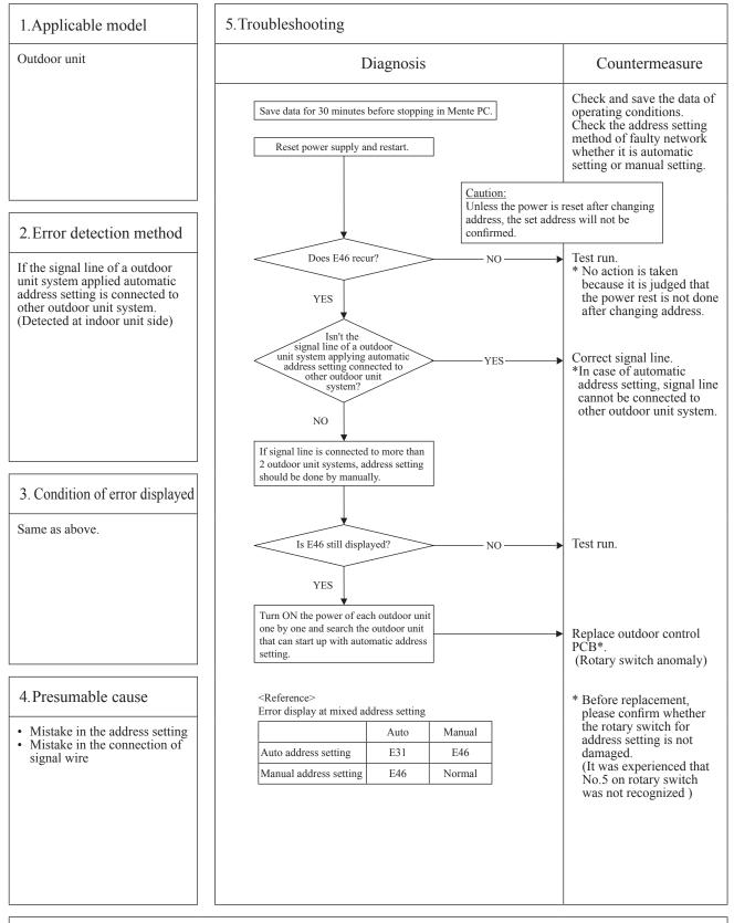
Note: After completing the above procedure, reset the power and confirm that the error display does not recur. Unless the power is reset for both indoor unit and outdoor unit, the set addresses will not be confirmed.
