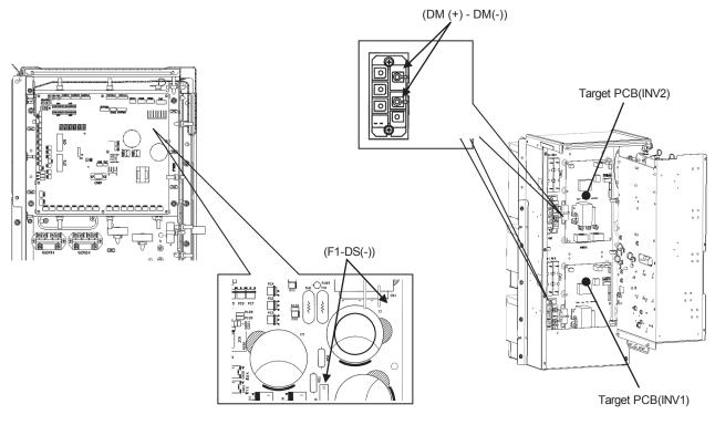
Fig.2 Voltage measurement points
