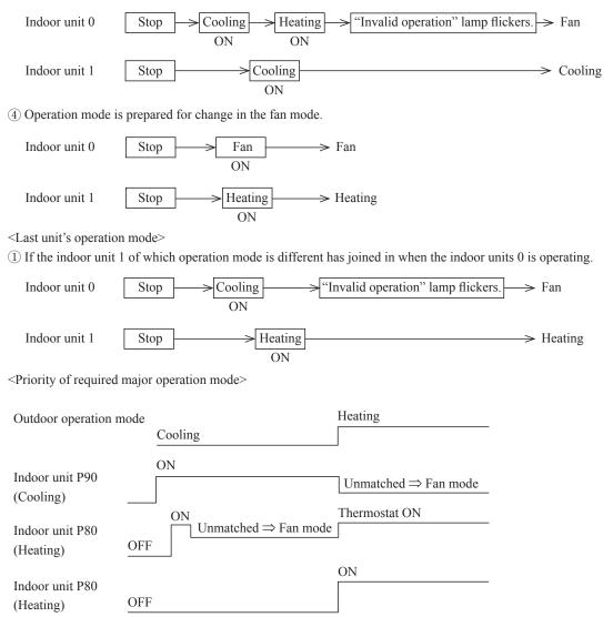
5) Reset of unmatched condition (Cooling/heating unmatched)
