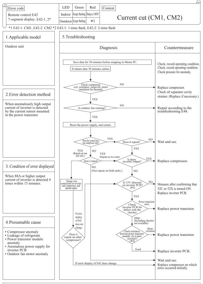
Note: \*3 Measurement position: Between + and - of C19 \*4 Measurement position: Check resistance between P-U, P-V, P-W, N-U, N-V, N-W, P-N. (Disconnect compressor wires before measurement.). If it fails to repeat, connect the Mente PC, and continue to collect data.
