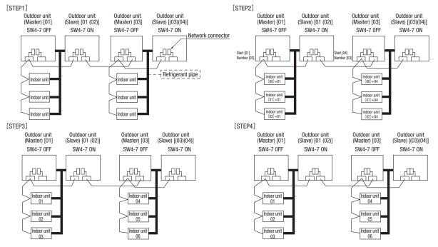
• Within a refrigerant system, indoor units are assigned addresses in the order they are recognized by the outdoor unit. Therefore, they are not necessarily assigned addresses in order from the nearest to the outdoor unit first as depicted in drawings above.
