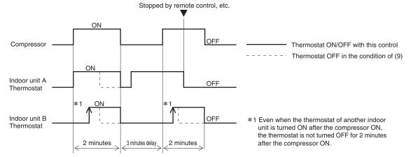
(b) When the oil return control has started while the thermostat is turned ON, the thermostat is not turned OFF even if the thermostat OFF condition is met during the oil return control.
