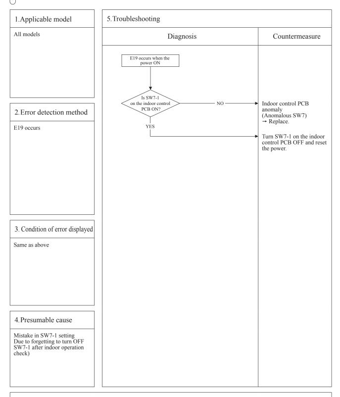
Note: Indoor operation check/drain pump check mode
