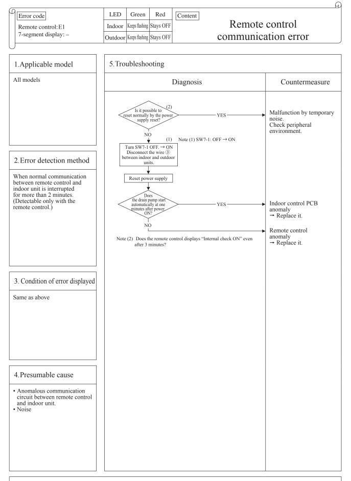
Note: If the indoor unit cannot communicate normally with the remote control for 180 seconds, the indoor unit PCB starts to reset automatically.
