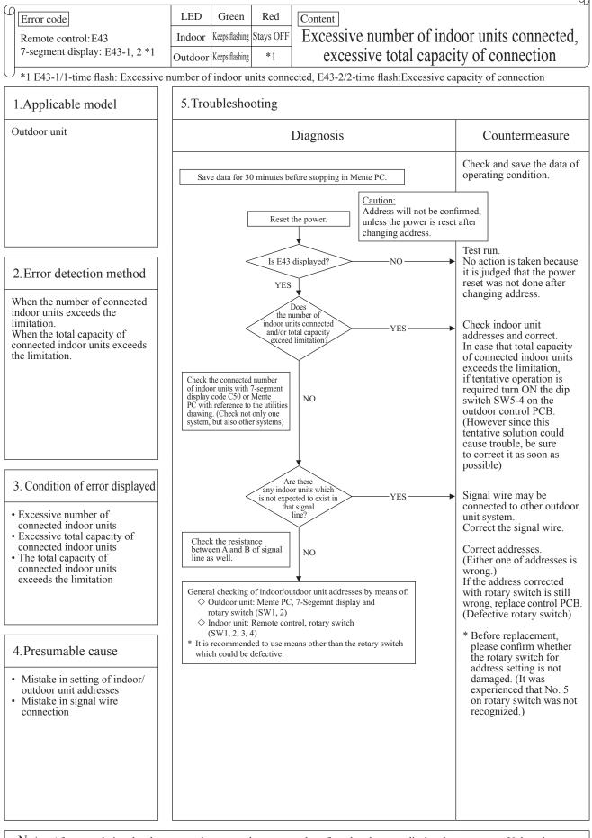
Note: After completing the above procedure, reset the power and confirm that the error display does not recur. Unless the power is reset for both indoor unit and outdoor unit, the set addresses will not be confirmed.
