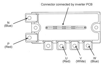
Fig.1 Parts arrangement view
