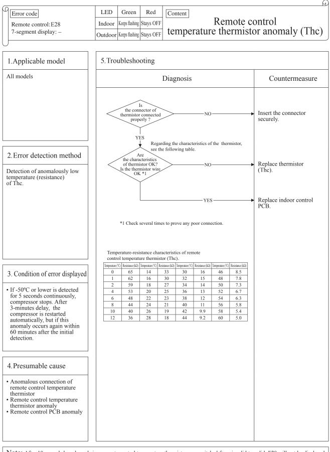
Note: After 10 seconds has elapsed since remote control temperature thermistor was switched from invalid to valid, E28 will not be displayed even if the thermistor harness is disconnected or broken. However, in such case, the indoor return air temperature thermistor (Thi-A) will be valid instantly instead of the remote control temperature thermistor (Thc).
