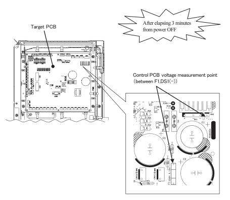
Fig.2 Voltage measurement points
