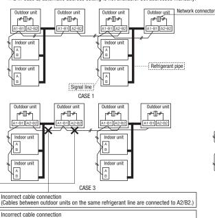
(Cables between outdoor units on different refrigerant lines are connected to A1/B1.)
