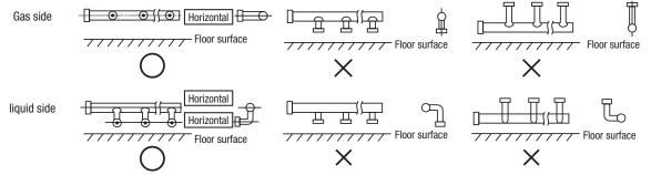
④ When using the outdoor unit's branch pipe set, make sure to secure a straight section of 500 mm or more for both the gas and liquid pipes before branching them.
