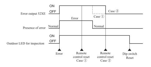
(c) The error output relay (52XE) is turned ON when the error stop occurs, and is turned OFF when the error reset is done from remote control by pressing "Check" and "Reset" button simultaneously after recovery from the error (Remote control reset case ②).
