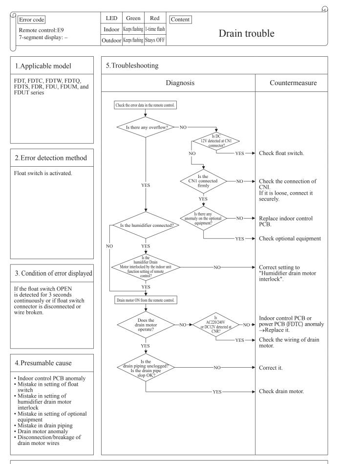
Note: When this anomaly occurs at power ON, disconnection of connector or breakage of wire of float switch is suspected. Check and correct it (or replace it, if necessary).
