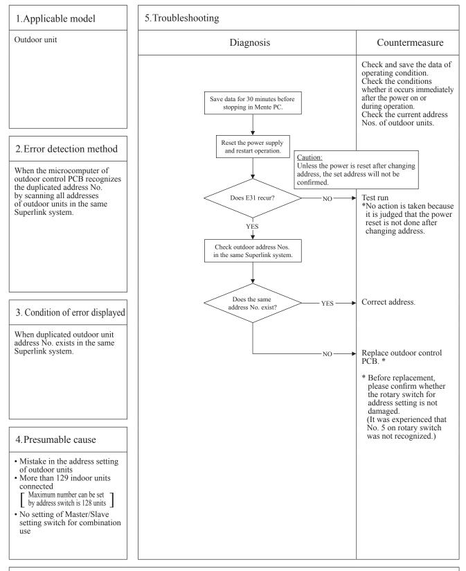
Note: After taken above measure, reset the power and confirm no error is displayed occurs. Unless the power is reset after changing address, the set address will not be confirmed. In case of combination use, set the same address to both master and slave units. Distinction of master or slave unit is done by setting SW4-7 and 4-8. (Refer the instruction manual and technical manual for details)
