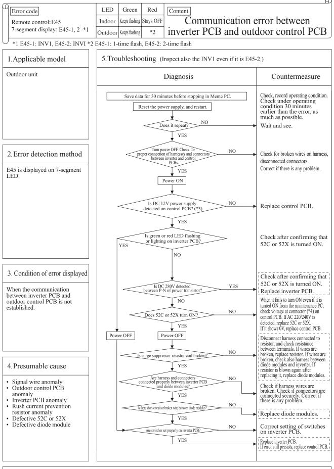
Note: \*3 Measurement position: Between + and - of C21 \*4 Measurement position: Between pins ① - ③ of CNM1, CNM2 (CNM2 for systems having 2 units of compressor only) If it fails to repeat, connect the Mente PC, and continue to collect data.
