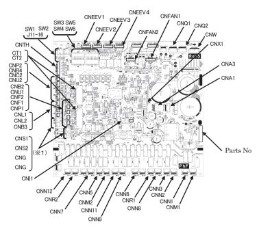
Fig.1 Parts arrangement
