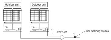
· Connect pipes between combined units, with care for the followings.
