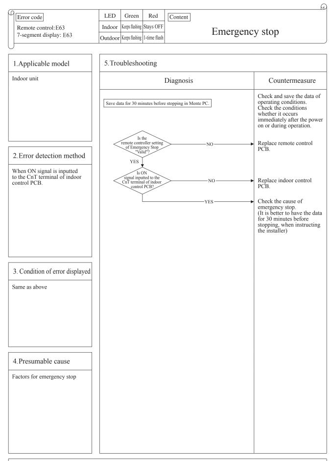
Note: Indoor unit detected emergency stop signal gives command "all stop"
