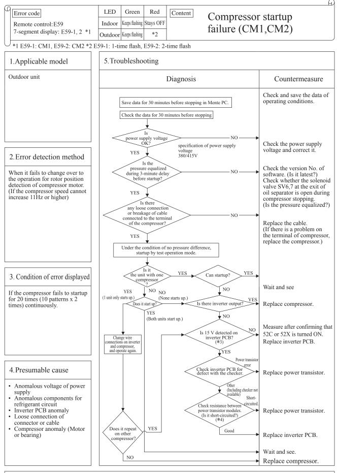
Note: \*3 Measurement position: Between + and - of C19 \*4 Measurement position: Check resistance between P-U, P-V, P-W, N-U, N-V, N-W, P-N. (Disconnect wires from compressor beforehand.) If it fails to repeat, connect the Mente PC, and continue to collect data.
