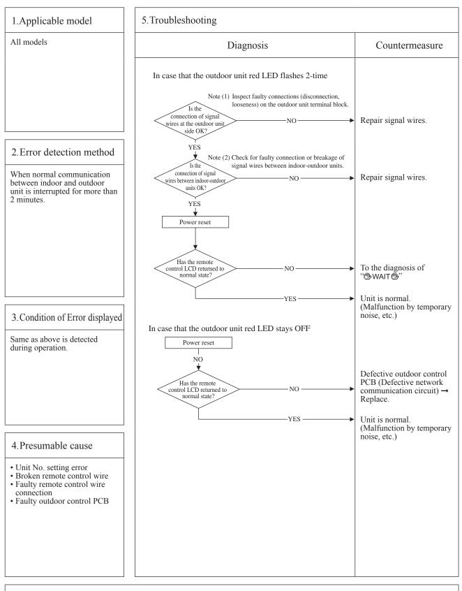
Note: Pressing the pump-down switch cancels communications between indoor and outdoor unit so that "communication error-E5" is displayed on indoor unit and remote control, but it is normal.
