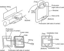
O Catch the two protrusion of the enclosed bracket onto the tting as shown above, and temporarily fix with the screws. (The bracket has an up/down and front/back orientation. Con rm the top/bottom protrusion positions and the positional relation of the ø 10 holes on the bracket and the installation hole on the lower case with the above drawing.)
