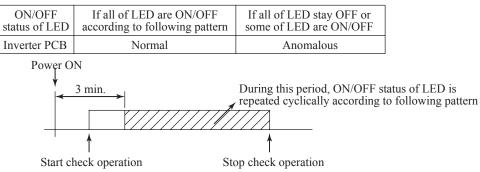
d) Stop check operation within about 2minutes after starting check operation.
