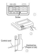
Prepare two M4 screws (recommended length is 12-16mm) on site, and install the lower case to erectrical box. Choose either of the following two positions in fixing it with screws.
