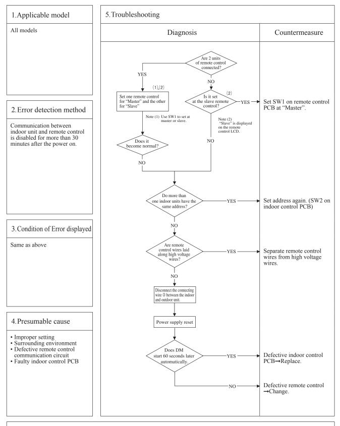
Note: If any error is detected 30 minutes after displaying "OWAITO" on the remote control, the display changes to "INSPECT I/U".
