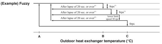
Notes (1) When the outdoor heat exchanger temperature is in the range of A~C°C, the speed is reduced by 8 rps at each 20 seconds.
