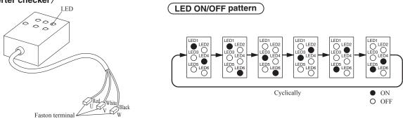
Connect to the terminal of the wires which are disconnected from compressor.
