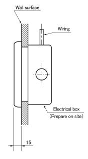
The remote control wiring can be extracted from the upper center. After the thin part in the upper side of the remote control upper case is scraped with a nipper or knife, remove burr with a file.
