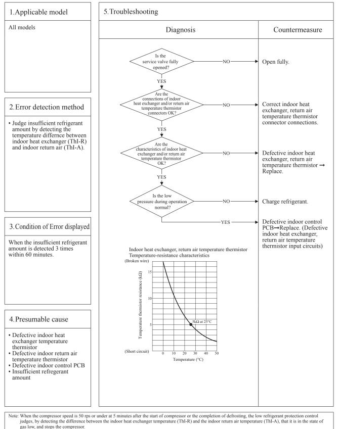
$\widetilde{Cooling}$ : Indoor return air temperature (ThI-A) – Indoor heat exchanger temperature (ThI-R)  $\ge 4$  deg Heating: Indoor heat exchanger temperature (ThI-R) – Indoor return air temperature (ThI-A)  $\le 6$  deg
