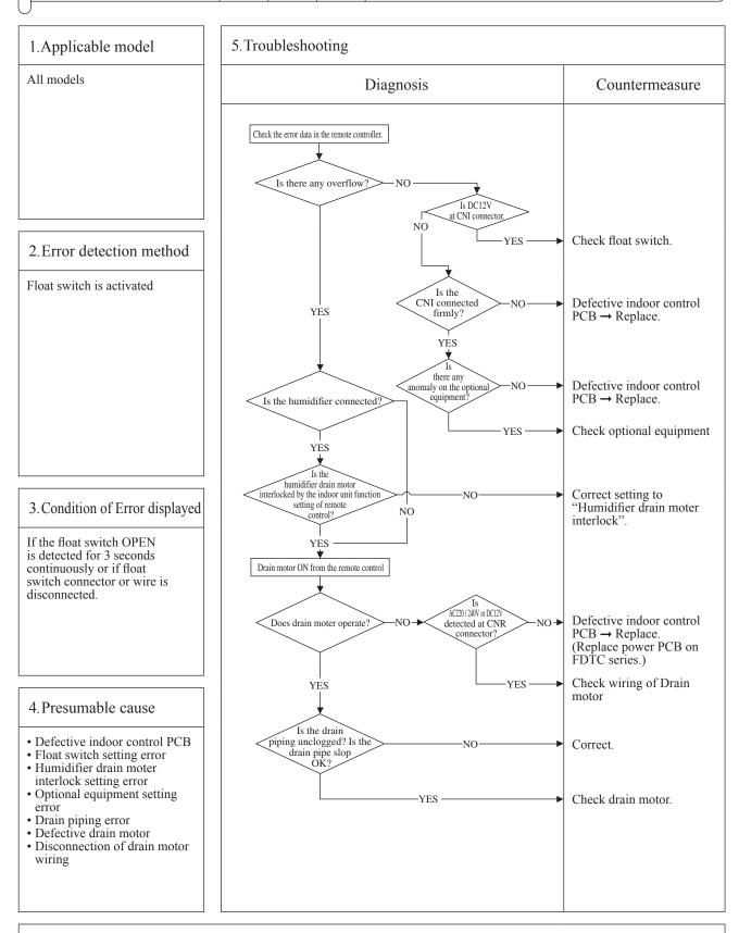
Note: When this error occurred at power ON, disconnection of wire or connector of the float switch is suspected. Check and correct it (or replace it, if necessary).
