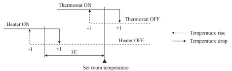
(iii) Thermostat is turned ON when the room temperature is in the range of -1 <Set point < +1 at the start of cooling operation (including from cooling to heating).
