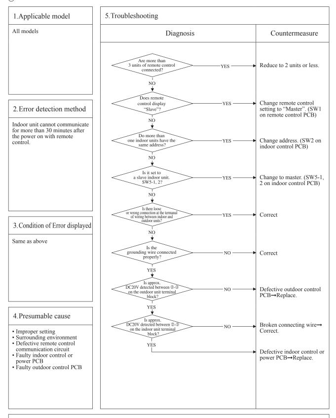
Note: If any error is detected 30 minutes after displaying ""WAIT"" on the remote control, the display changes to "INSPECT I/U".
