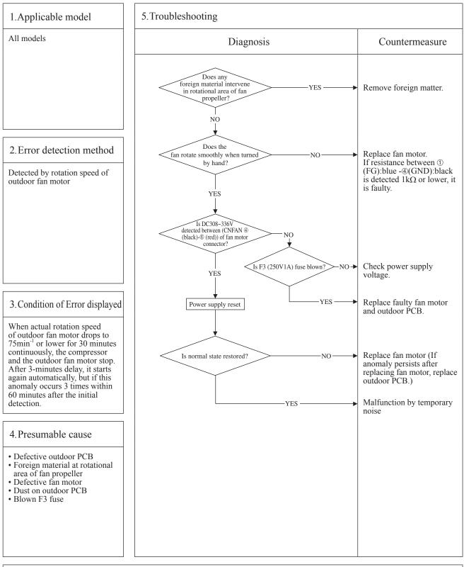
Note: When E48 error occurs, in almost cases F3 fuse (1A) on the outdoor PCB is blown. There are a lot of cases that fuse is blown and E48 occurs due to defective fan motor. And even though only the outdoor PCB ( or fuse) is replaced,, another trouble could occur. Therefore when fuse is blown, check whether the fan motor is OK or not. After confirming the fan motor normal, check by power ON. (Don't power ON without confirming the fan motor normal.)
