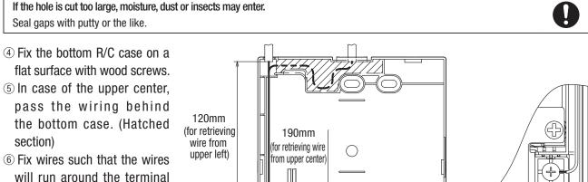
⑦ Install the top case with care not to pinch wires of R/C.
