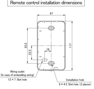
Note: Installation screw for remote control M4 Screw (2 pieces)
