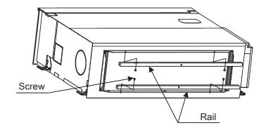
3) Install the air filter on the rails.
