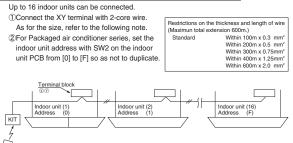
③For VRF series, set the indoor unit address with SW1, SW2 and SW5-2 on the indoor unit PCB from [000] to [127] so as not to duplicate
