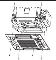
Tighten the panels to the brackets 3 and 4 with bolts. For further details, refer to the installation manual of panel.
