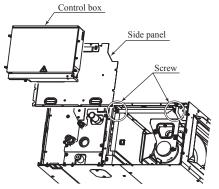
2) Take out the fan unit in the arrow direction.
