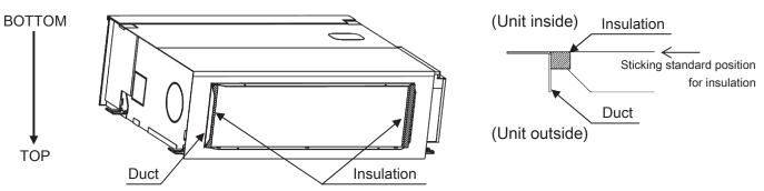
(\*) After unpacking, bottom side of the unit is located at the upper side.
