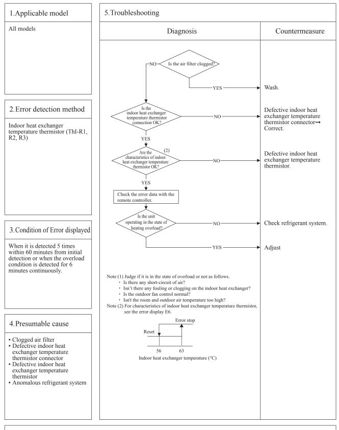
Note: During heating operation; After starting compressor, compressor rotation speed is decreased by detecting indoor heat exchanger temperature (ThI-R) in order to control high pressure.
