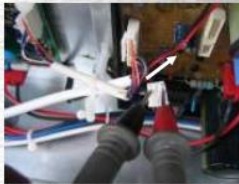
Measure the resistance of heat sink temperature sensor
