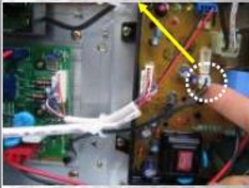
- Temperature sensor location of Heat sink
