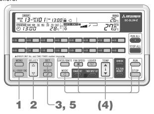
1. With normal running or stopping display (not in any setting mode \*), press the ALL / GROUP / ONE button and select either ALL | GROUP |, or ONE |.
