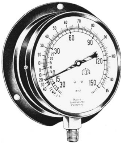
Fig. 1-22 This gage measures up to 150 psi pressure and also reads from 0 to 30 for vacuum. The temperature scaled runs from -40^{\circ} to 115^{\circ}\text{F} ( -40^{\circ} to 46.1^{\circ}\text{C} ).
