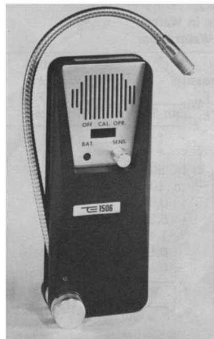
Fig. 6-5 A hand-held electronic leak detector. (Thermal Engineering)
