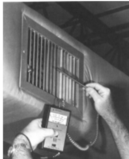
Figure 3-6. Proper use of an air velocity meter (Courtesy, Dwyer Instruments, Inc.)
