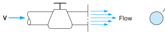
FIGURE 6.3 The flow across a control volume surface with a flow cross-sectional area of A . Average velocity is shown to the left of the valve and a distributed flow across the area is shown to the right of the valve.
