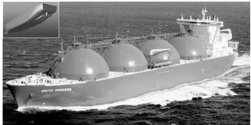
FIGURE 3.26 A tanker to transport liquefied natural gas (LNG), which is mainly methane.
