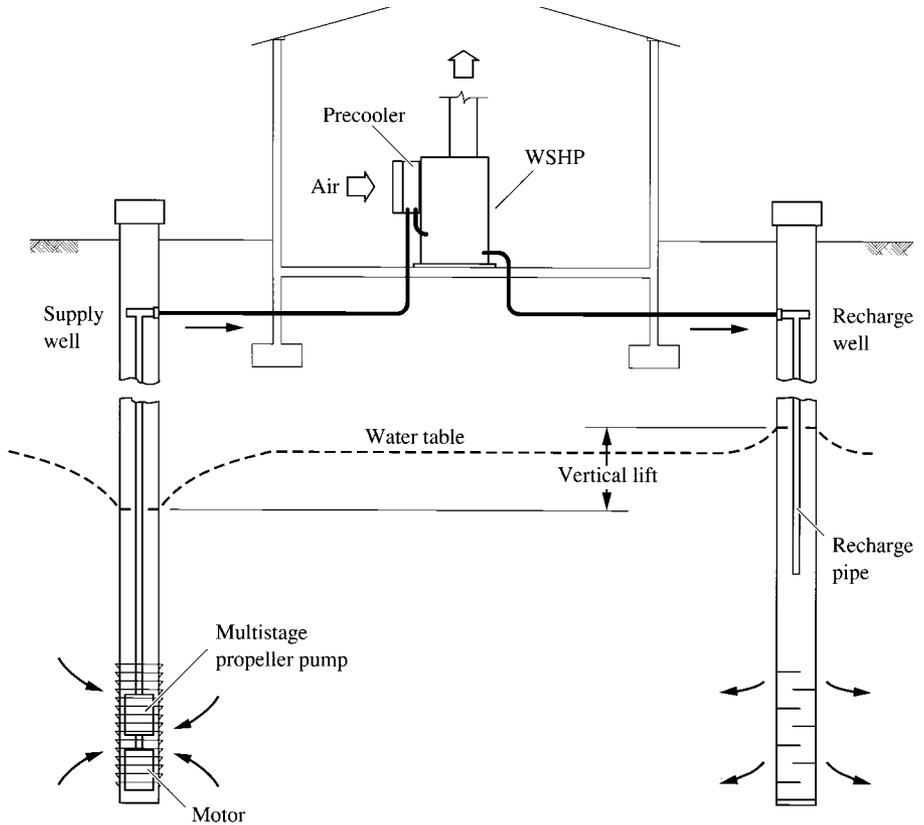
FIGURE 12.6 A typical residential groundwater heat pump system.
