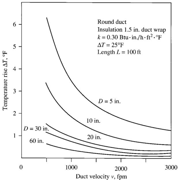
**FIGURE 17.5** Temperature rise curves from duct heat gain.
