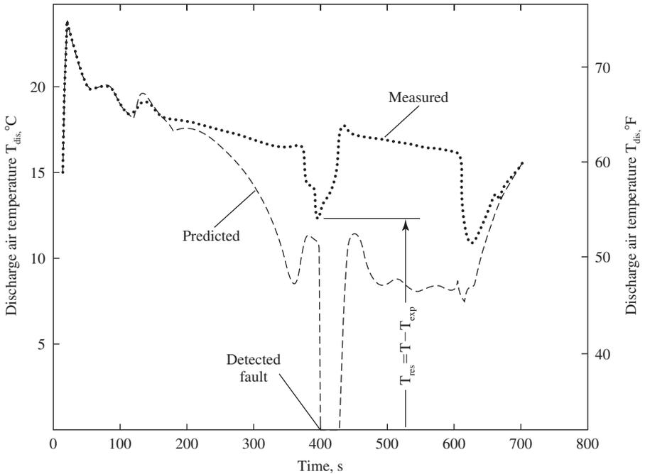
**FIGURE 5.27** Comparison of the measured and predicted discharge air temperatures for a VAV system in an ARX system model. (Source: Peitsman and Bakker (1996) *ASHRAE Transactions Part I* 6637. Reprinted with permission.)
