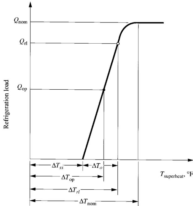
FIGURE 10.18 Capacity-superheat curve of a thermostatic expansion valve.
