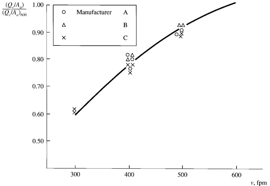
FIGURE 10.4 Variation of cooling capacity versus face velocity.
