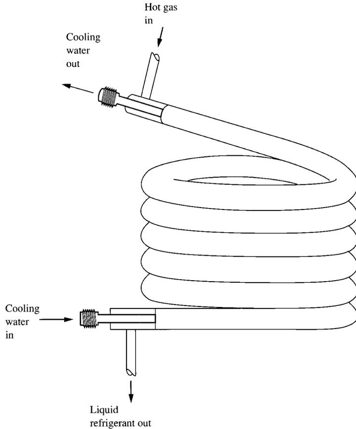
**FIGURE 10.9** Double-tube condenser.
