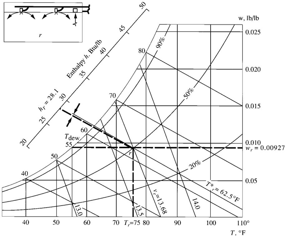
FIGURE 2.9 Thermodynamic properties determined from ASHRAE’s psychrometric chart.
