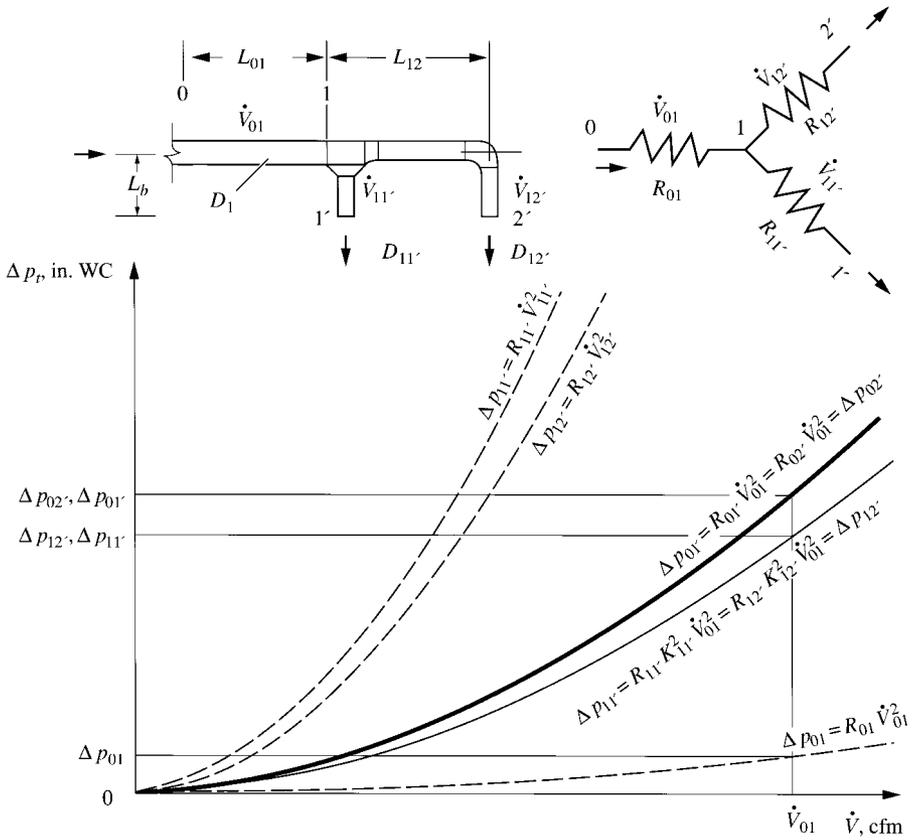
FIGURE 17.18 Flow resistance for a Y connection.
