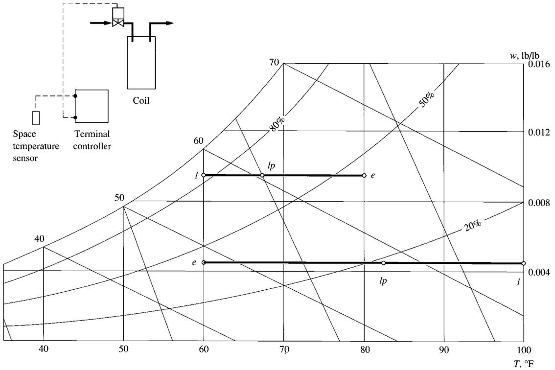
FIGURE 15.29 Dry coils at design and part-load operation.
