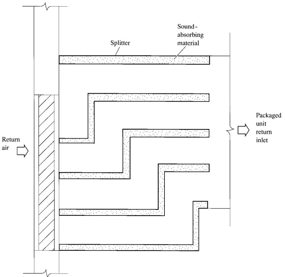
FIGURE 19.3 Sound-attenuating plenum.
