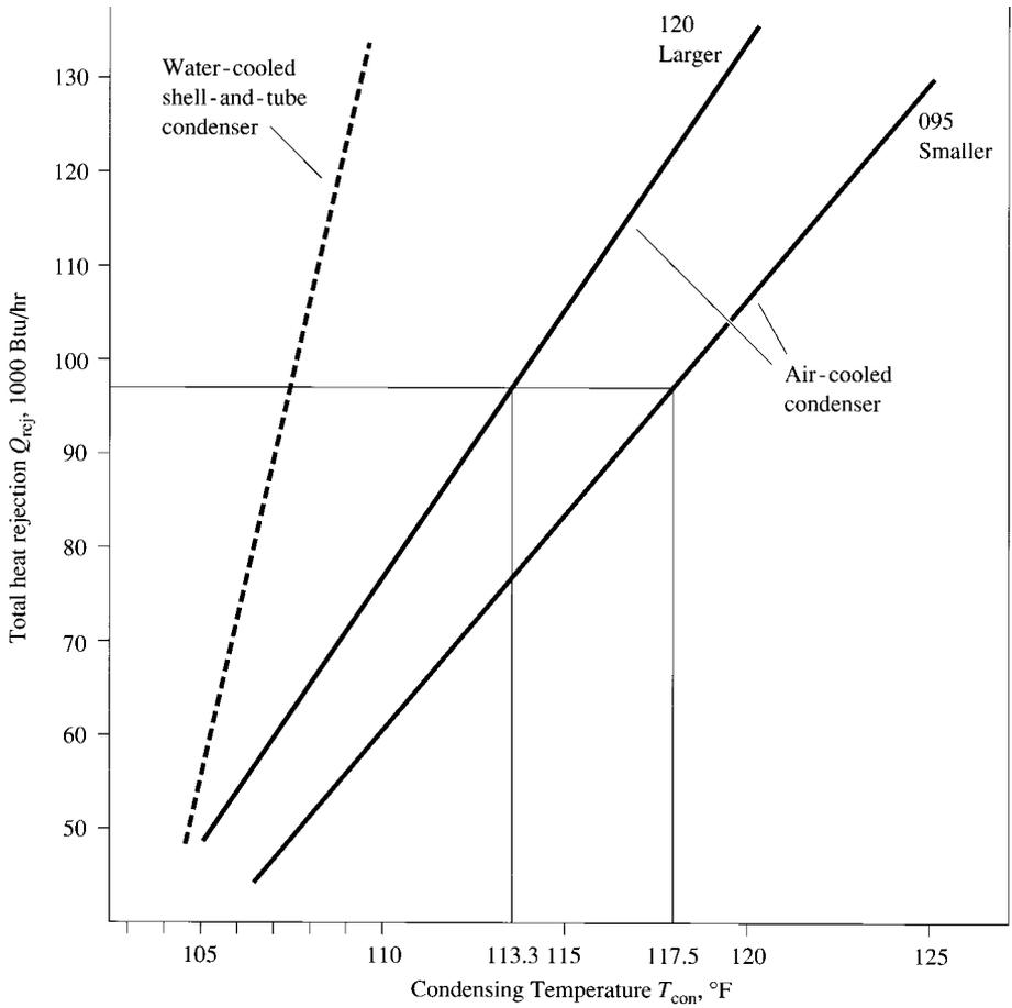
FIGURE 11.20 Performance curves  $Q_{rej}$ - $T_{con}$  for condensers.
