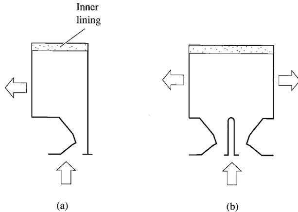
**FIGURE 18.13** Return slots: (a) single-slot; (b) double-slot.
