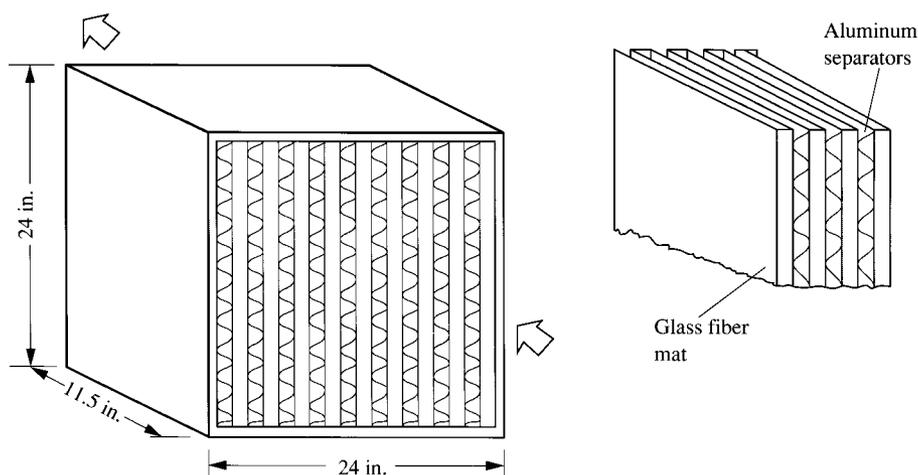
FIGURE 15.38 Ultrahigh-efficiency particulate filter (box filter).
