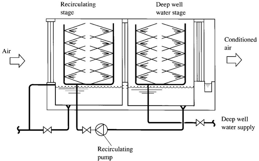
FIGURE 15.47 Two-stage air washer using deep well water.
