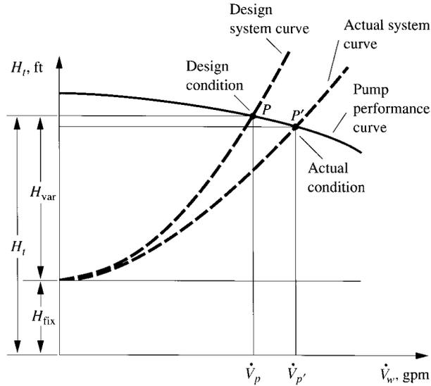
FIGURE 7.14 Water system curve and system operating point.
