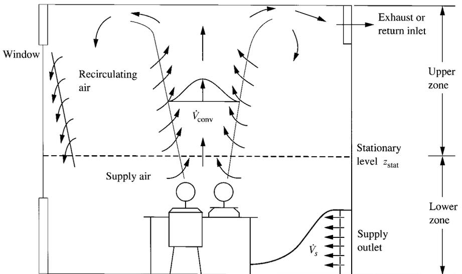
FIGURE 18.25 Stratified displacement flow in a typical room.
