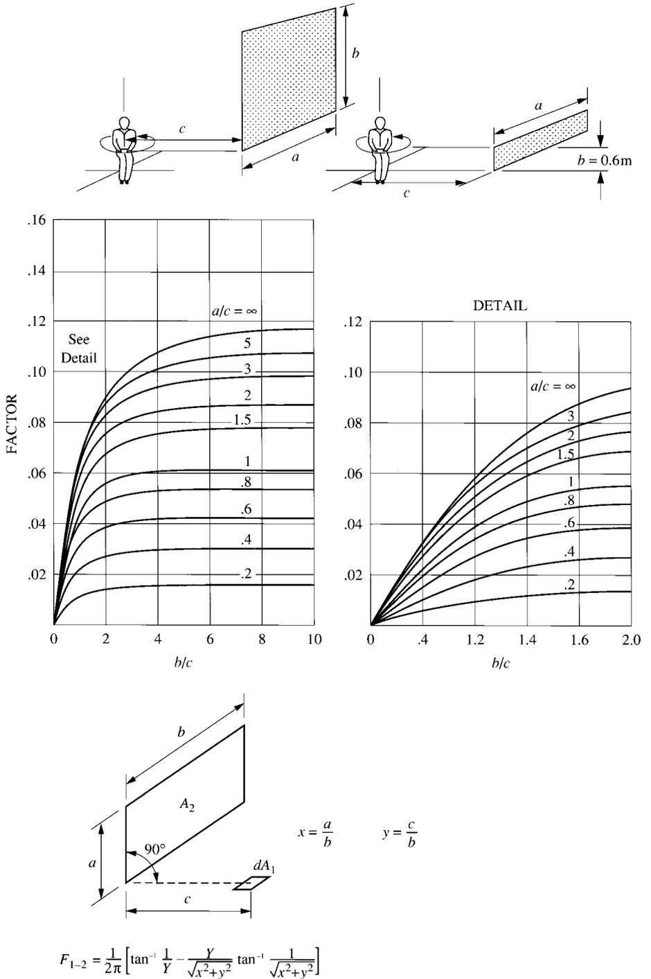
FIGURE 4.3 Mean value of shape factor between a seated person and a vertical plane. (Source: P. O. Fanger, *Thermal Comfort Analysis and Applications in Environmental Engineering*, 1970. Reprinted with permission.)
