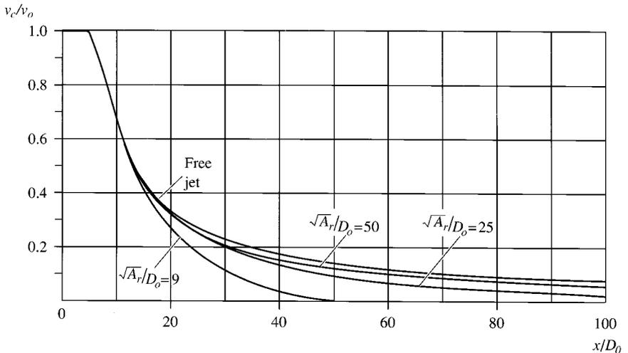
FIGURE 18.4 Centerline velocities of confined air jets.
