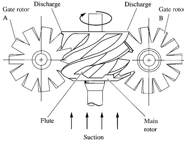
FIGURE 11.30 Single-screw compressor.
