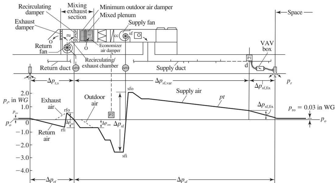
**FIGURE 22.1** System pressure diagram for a supply-return fan combination air system (connected in series) (rfi = return fan inlet; rfo = return fan outlet; sfi = supply fan inlet; sfo = supply fan outlet;  $\Delta p_{rf}$  = return fan total pressure;  $\Delta p_{sf}$  = supply fan total pressure; AFD = adjustable-frequency, variable-speed drive).
