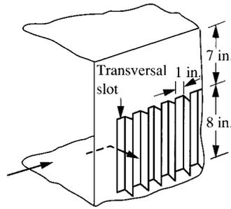
FIGURE 17.25 Rectangular supply duct with transversal slots.
