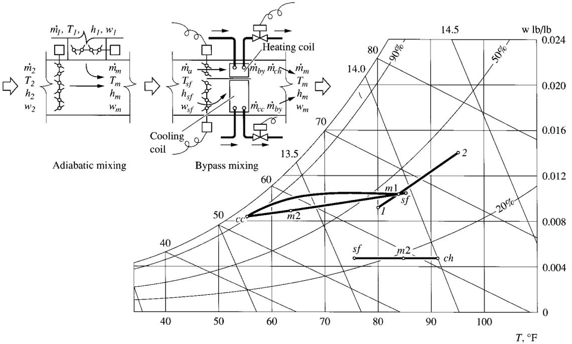
**FIGURE 20.21** Adiabatic mixing and bypass mixing processes.
