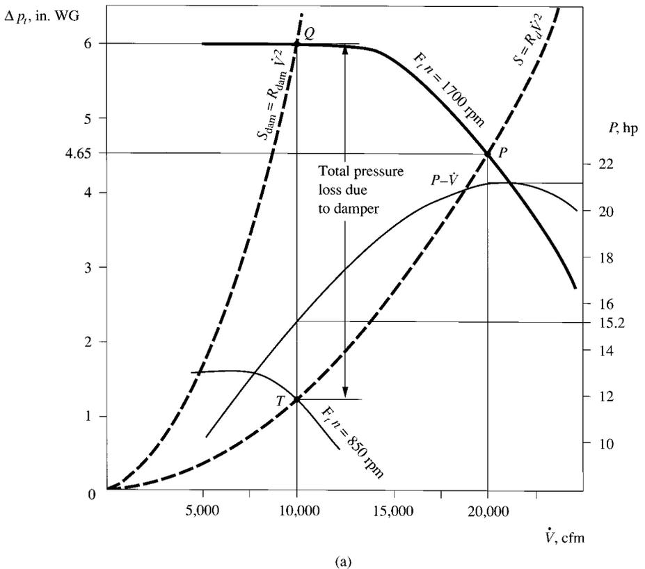
**FIGURE 20.15** Modulation of a VAV system using dampers, inlet vanes, and fan-speed variation: (a) using dampers and fan-speed variation; (b) using inlet vanes.
