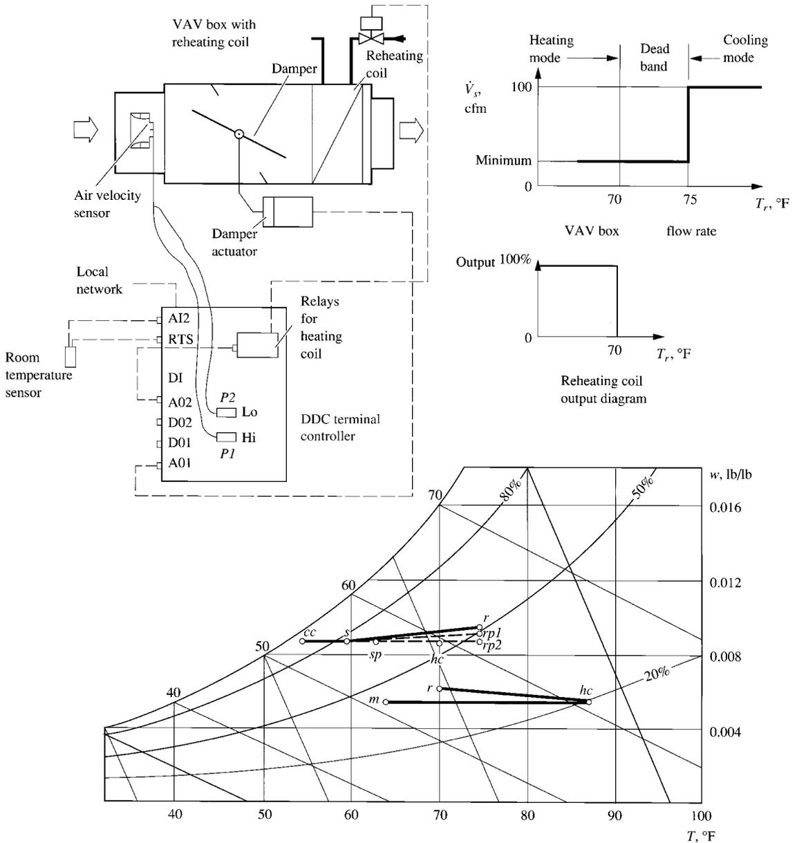
FIGURE 21.8 DDC for a reheating VAV box.
