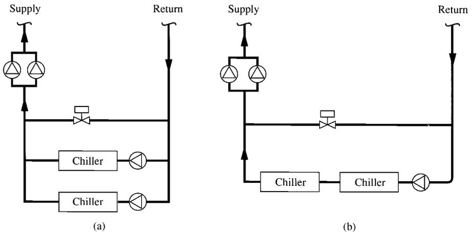
FIGURE 13.15 (a) Parallel chillers and (b) series chillers.
