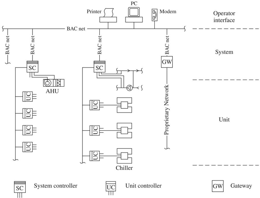
FIGURE 5.22 System architecture of a typical large EMCS.
