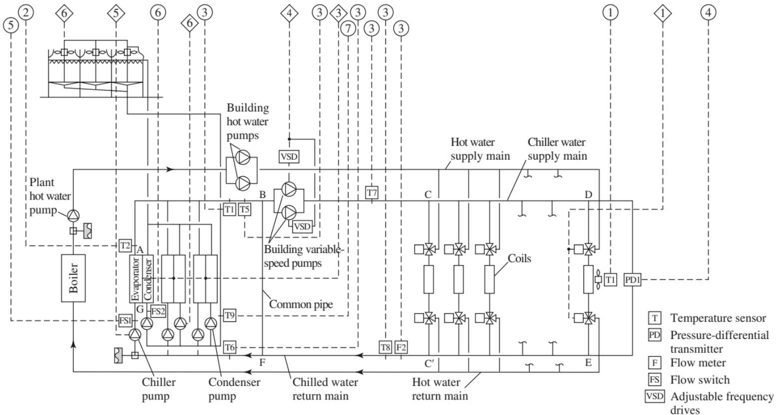
FIGURE 7.19 A dual-temperature water system with plant-building loop.
