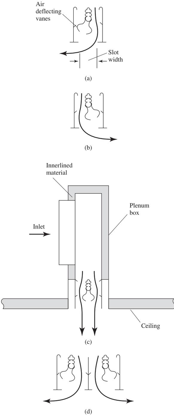
**FIGURE 18.9** Slot diffusers: (a) horizontal left; (b) horizontal right; (c) vertical; (d) two-slot, two-way.
