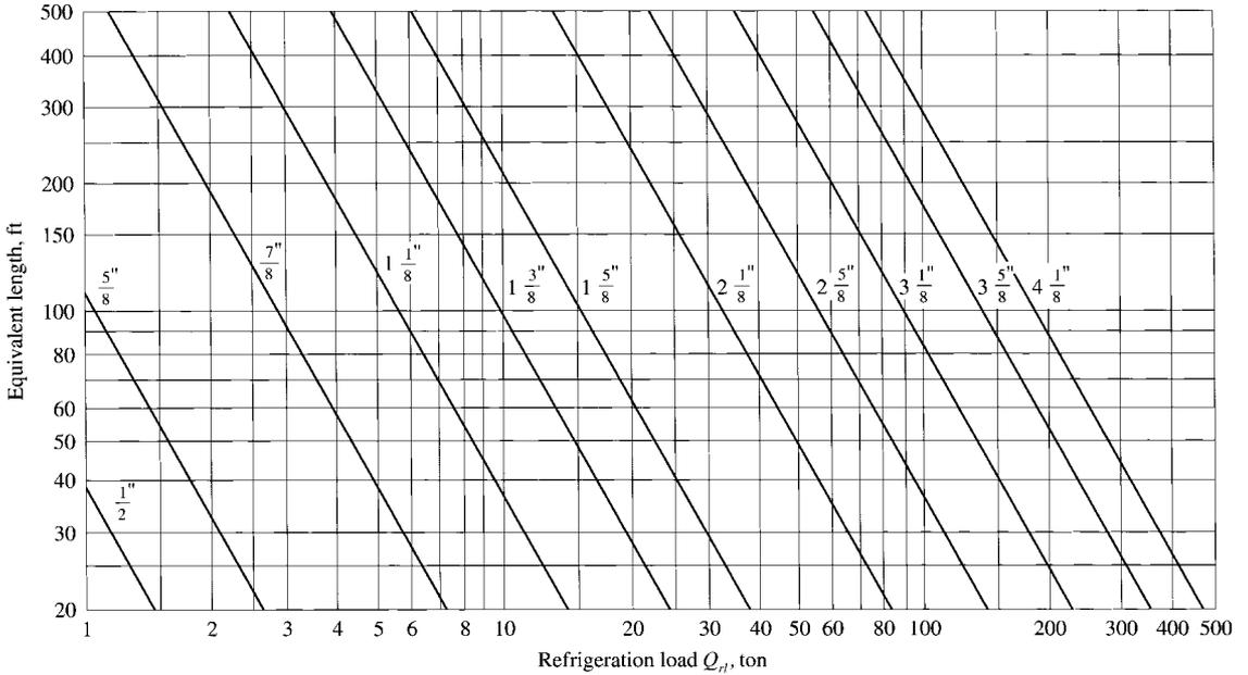
FIGURE 11.10 Suction line sizing  $Q_{rl}$ - $L_{eq}$  chart for HCFC-22 at 40°F suction temperature and 105°F condensing temperature (type L copper tube, outside diameter, 2°F change in saturated temperature).
