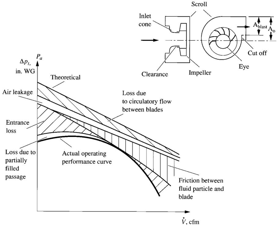
FIGURE 15.4 Operating characteristics for a backward-curved centrifugal fan.
