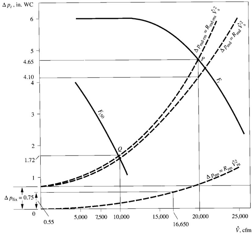
FIGURE 22.2 Air system of supply and exhaust fan combination: (a) schematic diagram; (b) system characteristics on  $\Delta p_t - \dot{V}$  diagram.
