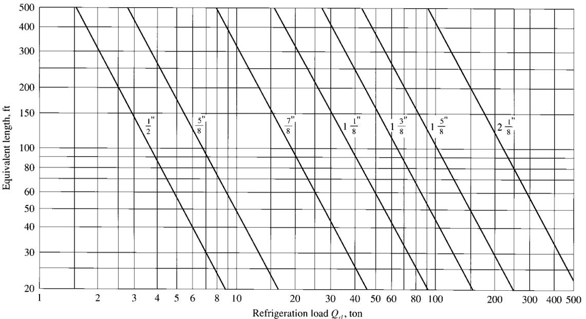
FIGURE 11.12 Liquid line sizing  $Q_{rl}-L_{eq}$  chart for HCFC-22 at 40°F suction temperature and 105°F condensing temperature (type L copper tube, outside diameter, 1°F change in saturated temperature).
