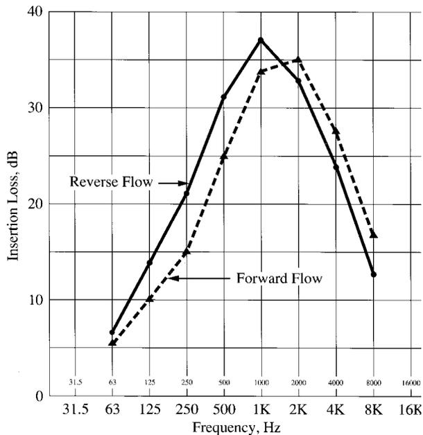
**FIGURE 19.4** Difference in insertion loss of a rectangular silencer between forward and reverse flow (at 2000 fpm or 10 m/s face velocity). (Source: *Handbook of HVAC Design*, 1990. Reprinted by permission.)
