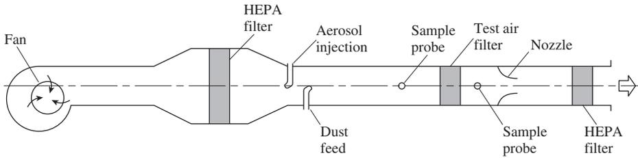
FIGURE 15.36 ANSI/ASHRAE Standard 52.2 specified air filter test unit.
