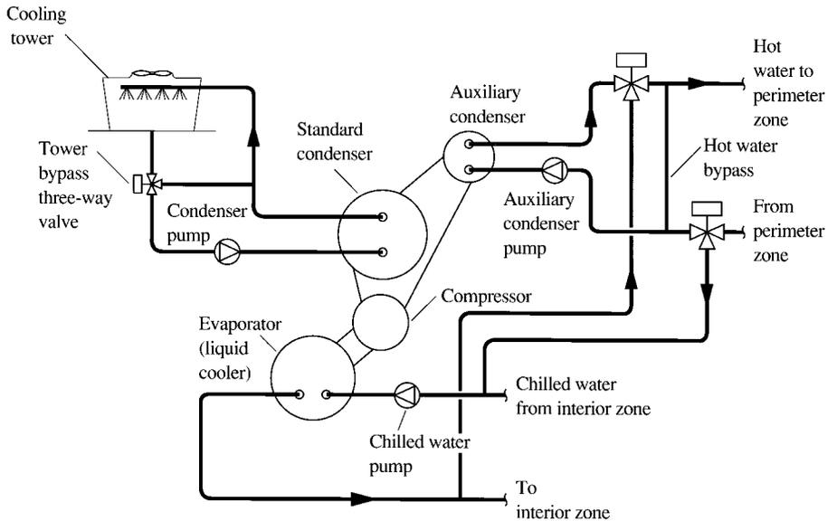
FIGURE 13.6 Heat recovery system using an auxiliary condenser.
