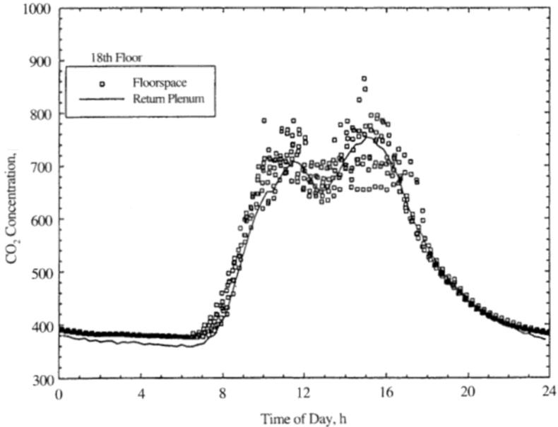
**FIGURE 23.1** CO<sub>2</sub> concentration profiles measured in the floor space and in the return air duct on the 18th floor with minimum 20 percent outdoor air supply. *Source: Reardon et al., ASHRAE Transactions, Part II, 1994*
