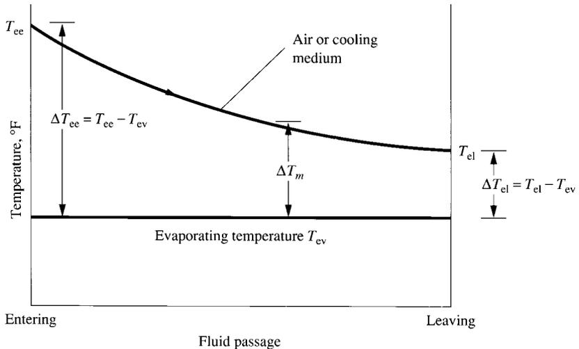
**FIGURE 10.6** Heat-transfer process in a flooded shell-and-tube cooler.
