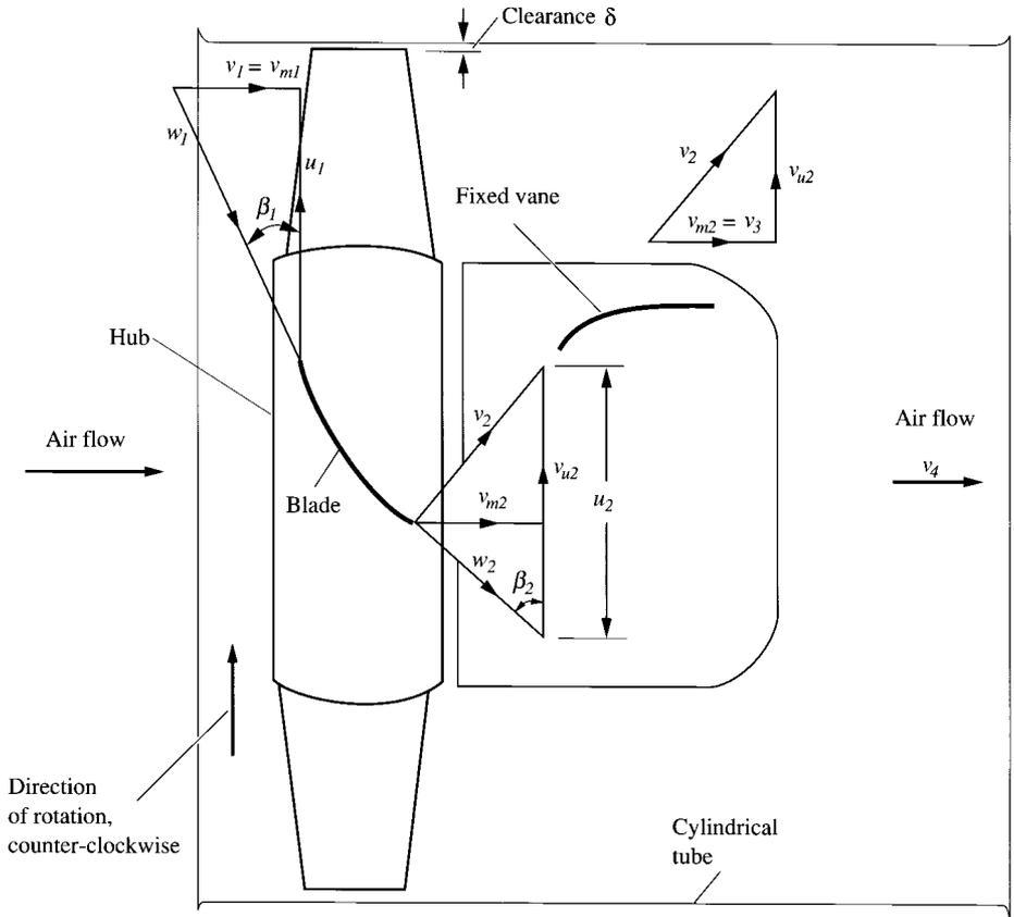
FIGURE 15.12 Velocity triangles for a vane-axial fan.
