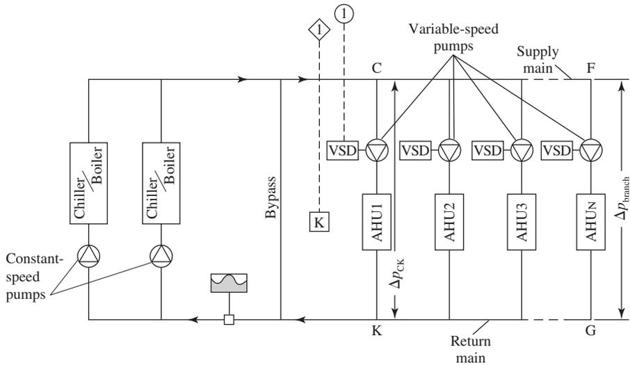
FIGURE 7.21 Schematic diagram of a plant-distributed pumping loop .
