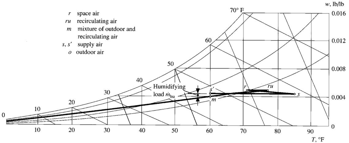
FIGURE 15.41 Humidifying load for a typical air system.
