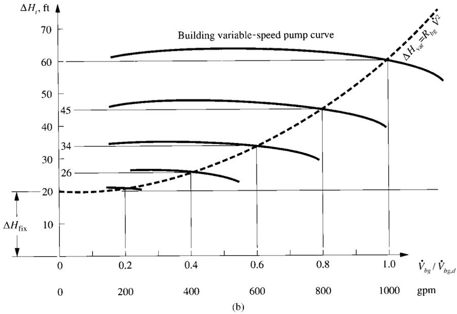
**FIGURE 7.20** System performance curves for plant-building loop. (a) Schematic diagram; (b) head of building variable-speed pump at various volume flow rates; (c)  $\dot{V}_{bg}$  versus  $Q_{cs}/Q_{cs,d}$  and  $\dot{V}_{bg}/\dot{V}_{bg,d}$  versus  $Q_{cs}/Q_{cs,d}$ ; (d)  $\Delta T_{w,c}$  versus  $Q_{cs}/Q_{cs,d}$ .
