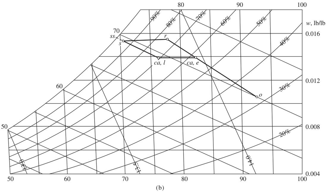
**FIGURE 27.4** Operating characteristics of an indirect-direct two-stage evaporative cooling system: (a) using outdoor air as cooled air and wet air; (b) using 30 percent outdoor air and 70 percent recirculating air mixture as cooled air and return air as wet air.
