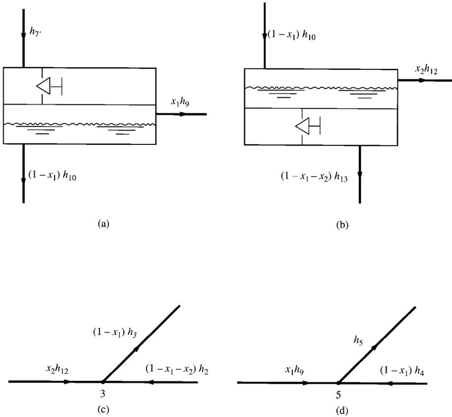
**FIGURE 9.10** Heat balance of refrigerants entering and leaving the high-pressure and low-pressure flash cooler and mixing points. (a) High-pressure flash cooler; (b) low-pressure flash cooler; (c) at the mixing point before entering second-stage impeller; (d) at the mixing point before entering third-stage impeller.
