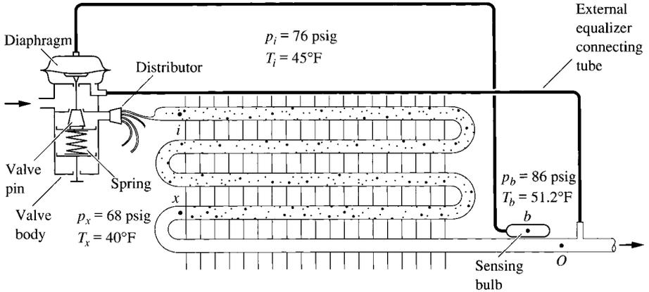
FIGURE 10.17 Thermostatic expansion valve with external equalizer.
