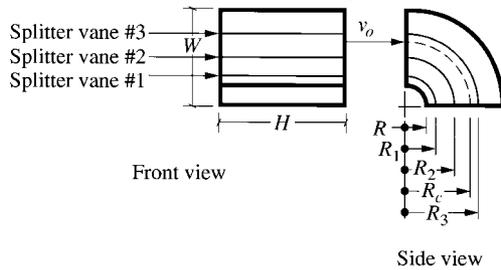
Coefficients for elbows with two splitter vanes  $C_o$
