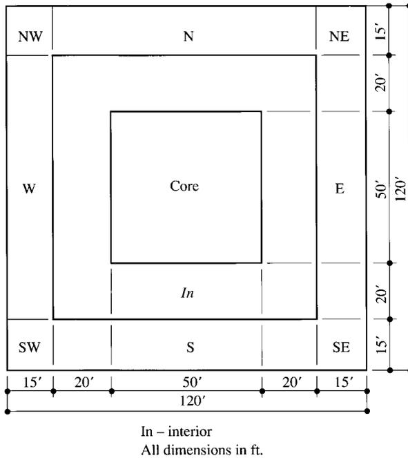
FIGURE 6.9 Typical plan of a high-rise office building.
