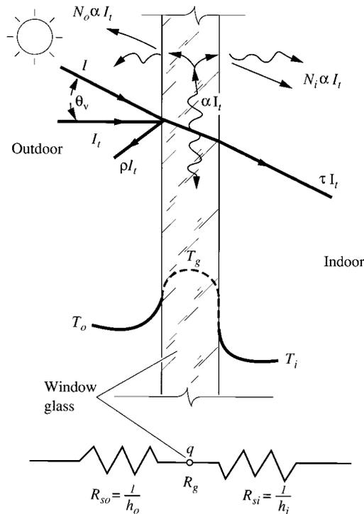
FIGURE 3.11 Heat admitted through a single-glazing window glass.
