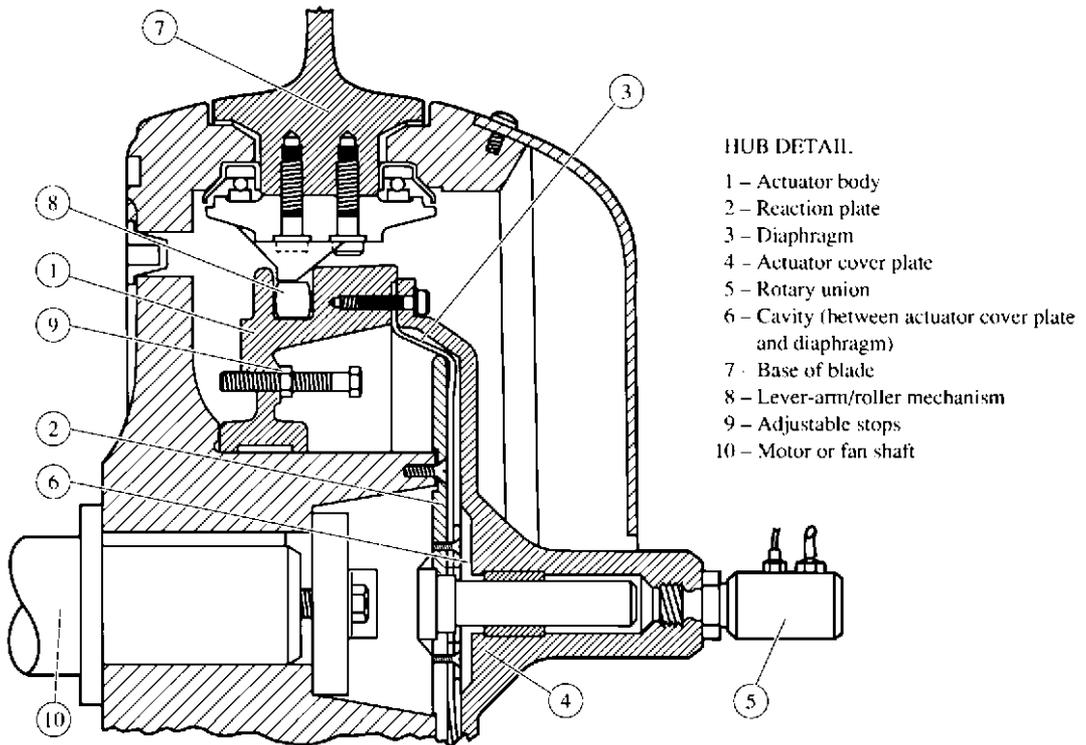
FIGURE 15.19 Controllable-pitch vane-axial fan blade pitch control mechanism.
