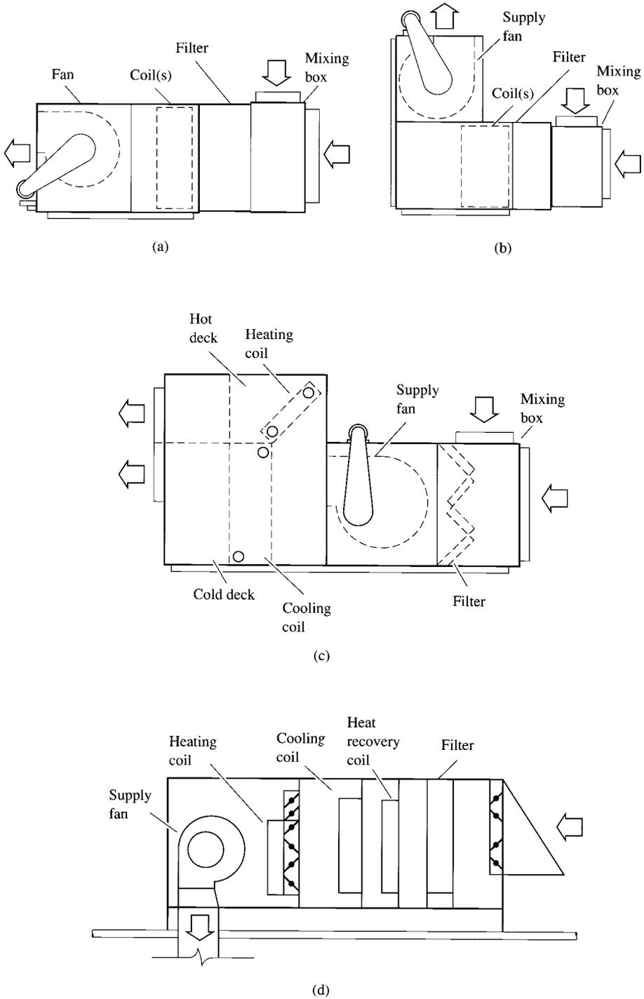
**FIGURE 16.1** Type of air-handling units (AHUs): (a) horizontal, draw-through unit; (b) vertical draw-through unit; (c) blow-through unit, multizone AHU; (d) makeup air AHU, custom-built, rooftop unit.
