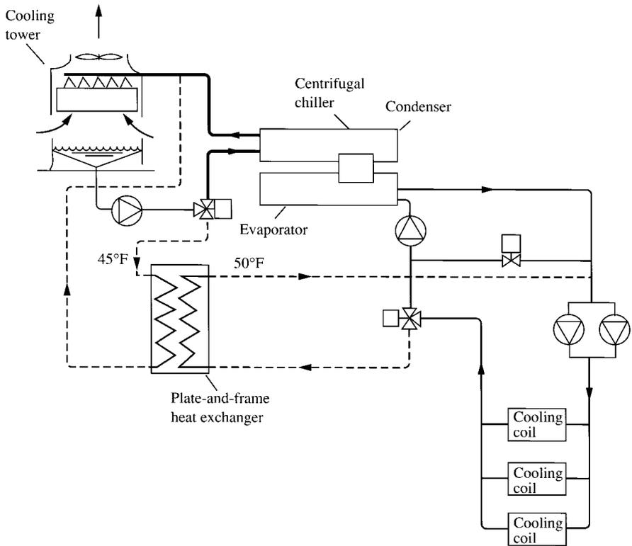
**FIGURE 27.7** Tower, plate-and-frame heat exchanger, and coil combination.
