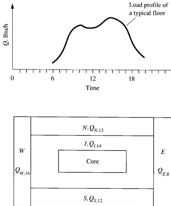
FIGURE 6.5 Load profile, peak load, and block load.
