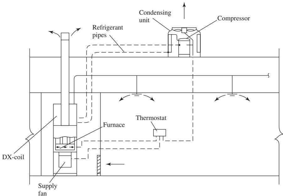
FIGURE 5.1 A single-zone, two-position electric control system.
