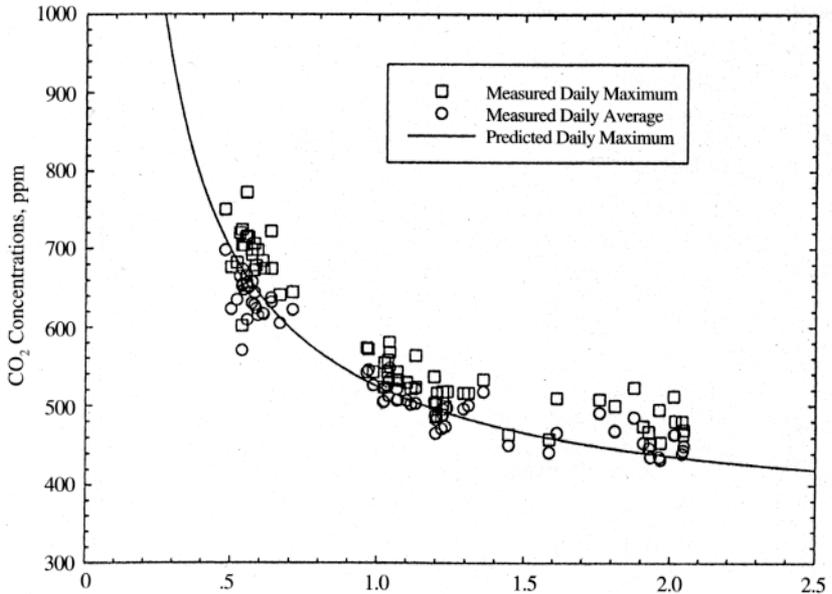
**FIGURE 23.2** Measured daily peak and daily average CO<sub>2</sub> concentrations in the return duct versus air changes per hour. (Source: Reardon et al., *ASHRAE Transactions, Part II, 1994*)
