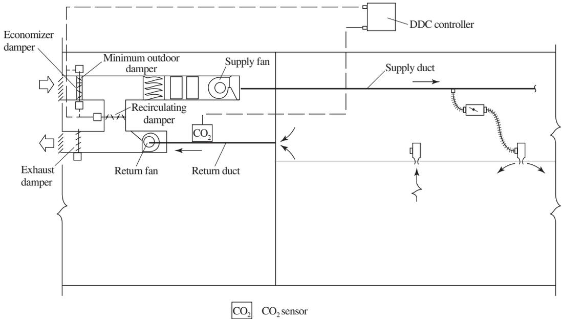
FIGURE 23.3 A CO<sub>2</sub>-based demand-controlled ventilation control in a VAV system.
