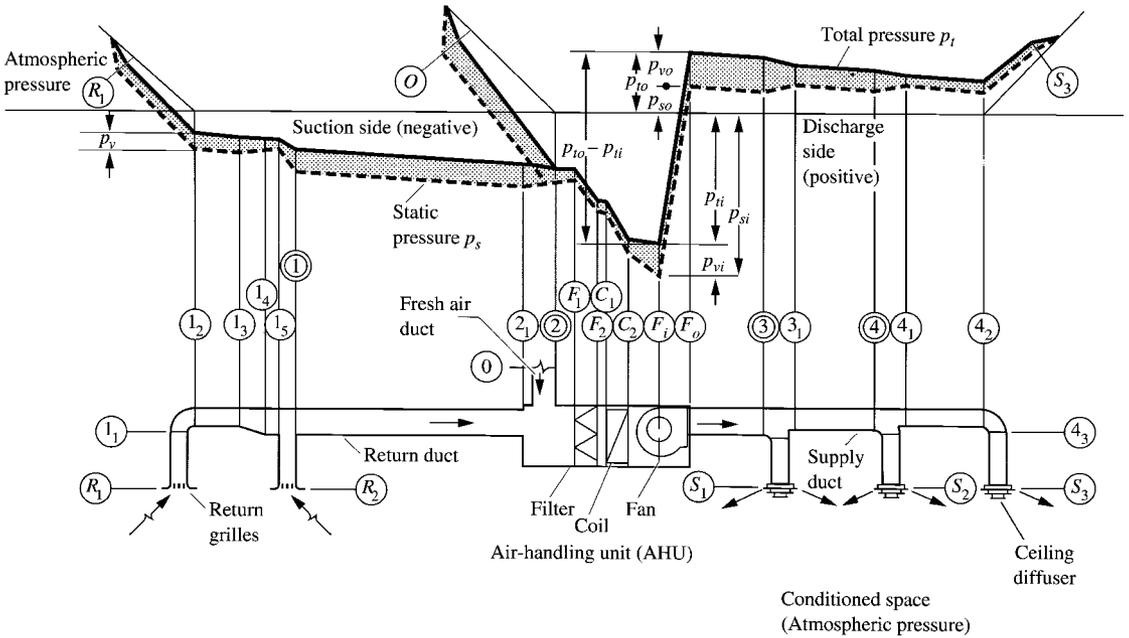
FIGURE 17.3 Pressure characteristics of a fan duct system.
