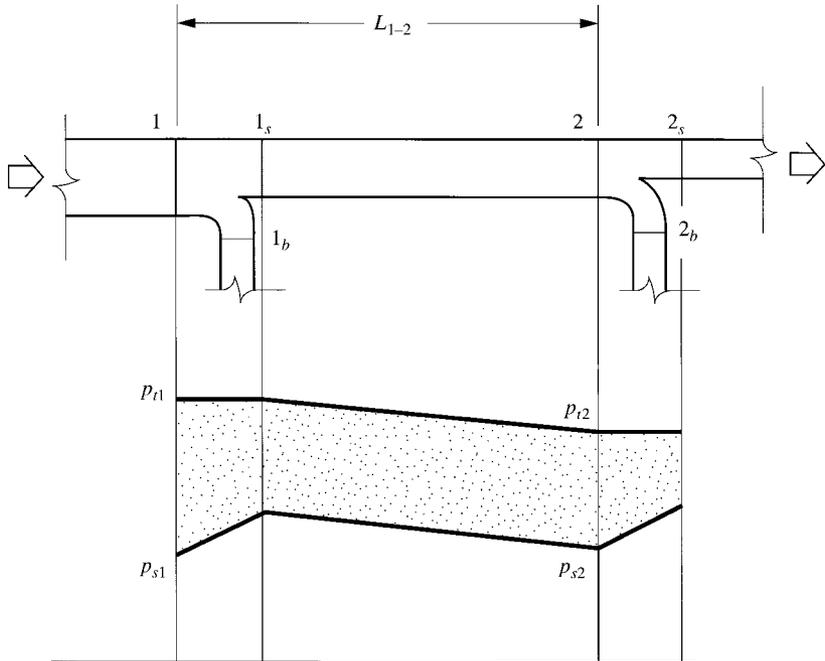
FIGURE 17.22 Pressure characteristics of a main duct section.
