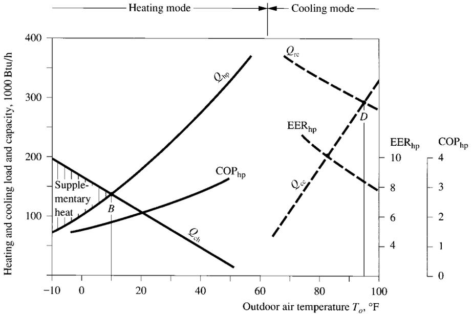
FIGURE 12.4 System performance of a rooftop heat pump.
