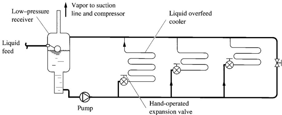
FIGURE 10.8 Liquid overfeed cooler using a mechanical pump.
