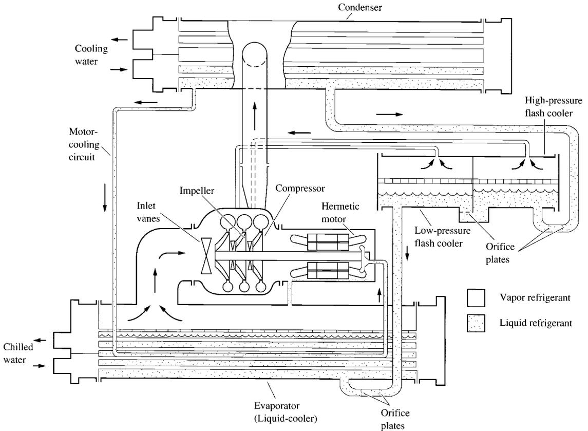
FIGURE 13.1 A typical three-stage, water-cooled centrifugal chiller.
