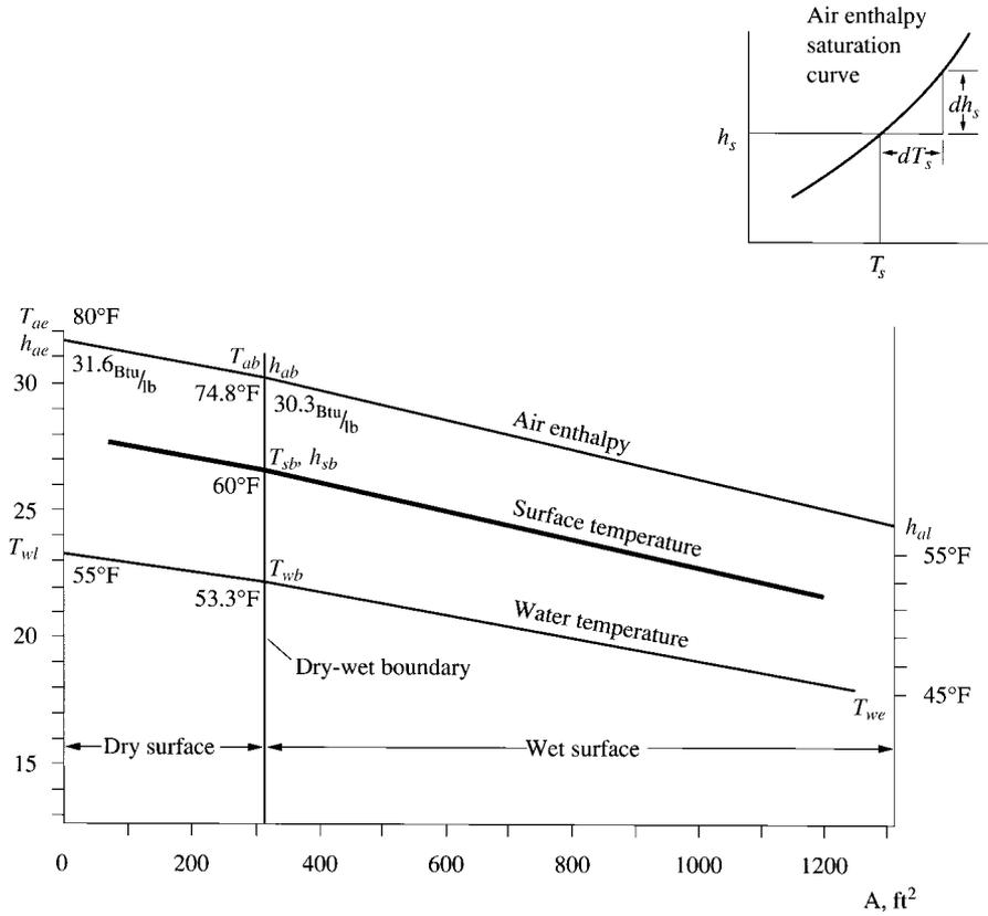
FIGURE 15.31 Dry-wet boundary of a dry-wet coil.
