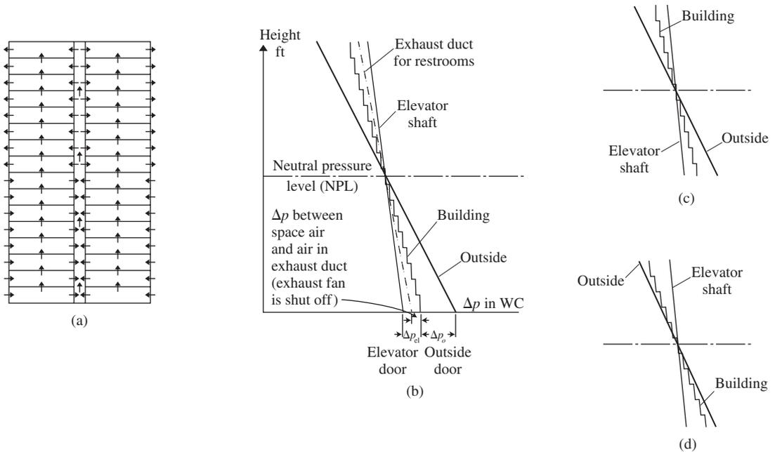
**FIGURE 20.1** Stack effect in a high-rise building (a) schematic diagram of building airflow; (b) pressure profiles; (c) pressure profiles for tight building shell; (d) pressure profiles for leaky building shell.
