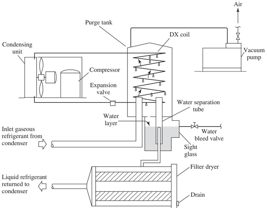
FIGURE 13.4 A purge unit in a centrifugal chiller.
