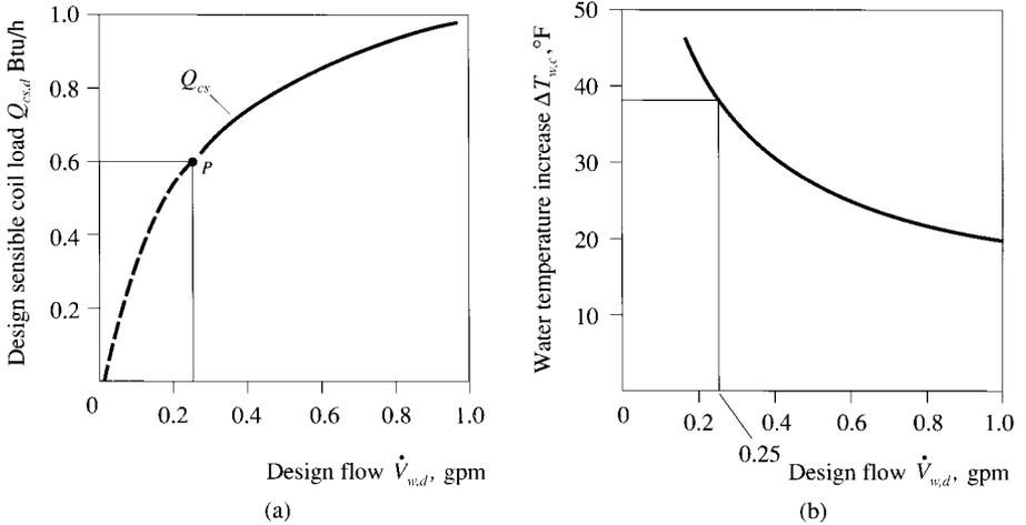
**FIGURE 7.17** Relationship between fraction of design volume flow rate  $\dot{V}_{w,d}$ , coil load  $Q_{cs}$ , and water temperature rise  $\Delta T_{wc}$ . (a)  $Q_{cs}$  versus  $\dot{V}_{w,d}$ ; (b)  $\Delta T_{wc}$  versus  $\dot{V}_{w,d}$ .
