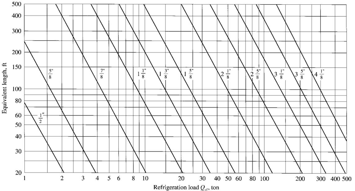
**FIGURE 11.11** Discharge line sizing  $Q_{rl}$ - $L_{eq}$  chart for HCFC-22 at 40°F suction temperature and 105°F condensing temperature (type L copper tube, outside diameter, 1°F change in saturated temperature).
