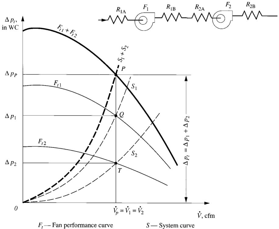
FIGURE 20.9 Two-fan fan-duct system connected in series.
