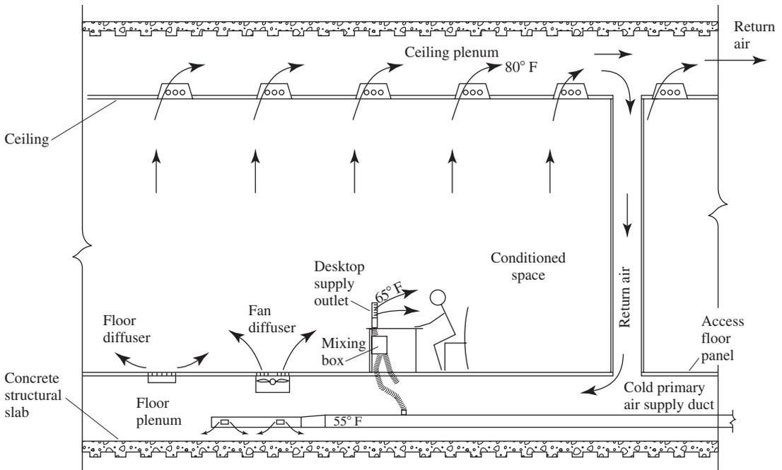
FIGURE 18.27 Upward flow underfloor air distribution system.
