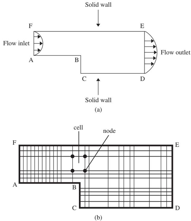
**FIGURE 18.28** Calculation of airflow using CFD in a duct section: (a) a duct section with sudden expansion; (b) finite element model for airflow in a duct section. (Source: ASHRAE Journal, January 1997. Authors Ladeinde and Neeron. Reprinted by permission.)
