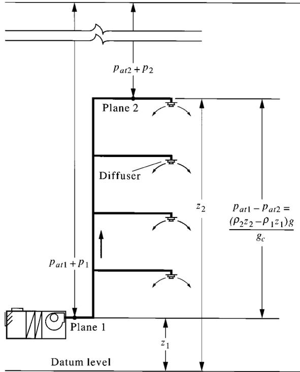
FIGURE 17.1 Pressure characteristics of an air duct system.
