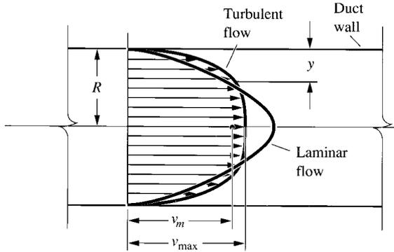
FIGURE 17.2 Velocity distribution in a circular duct.
