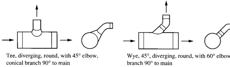
Tee, diverging, round, with 45° elbow, conical branch 90° to main
