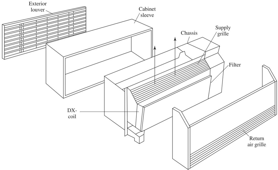
FIGURE 26.2 A packaged terminal air conditioner.
