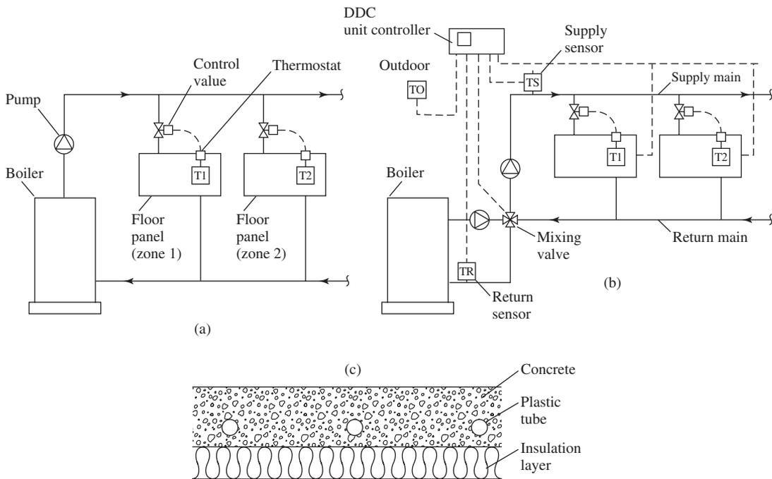
**FIGURE 8.9** Hydronic radiant floor heating systems. (a) Zone control valves; (b) outdoor reset plus zone control valves; (c) floor panel; (d) design nomograph. (Source: *ASHRAE Transactions 1995 Part I*, p. 1204, Kilikis and Coley. Reprinted by permission.)
