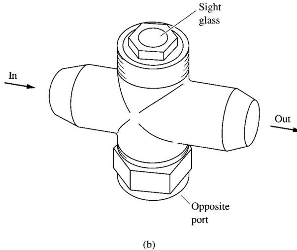
FIGURE 11.7 (a) Filter dryer and (b) sight glass.
