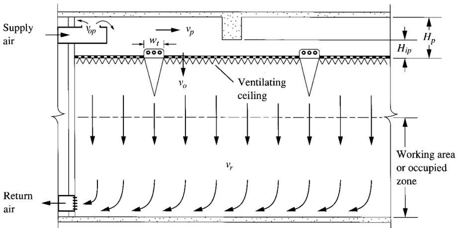
FIGURE 18.24 Ventilating ceiling.
