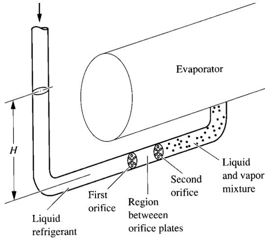
FIGURE 13.3 Orifice plates.
