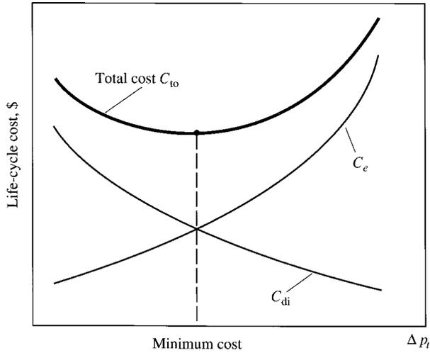
**FIGURE 17.23** Cost analysis for a duct system.
