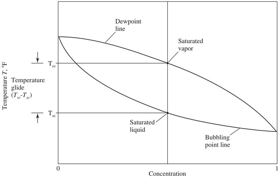
FIGURE 11.27 Temperature-concentration diagram of a zeotropic refrigerant blend.
