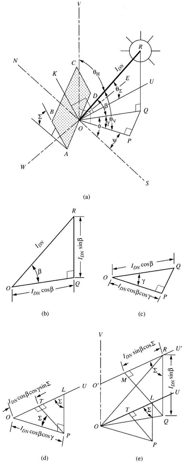
FIGURE 3.7 Solar intensity and angle of incidence.
