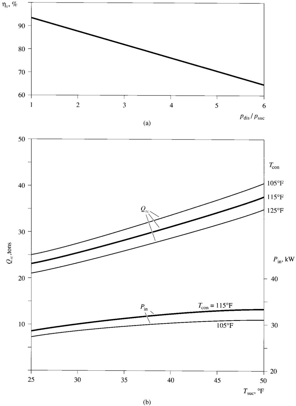
**FIGURE 11.18** Cooling capacity, power input, and volumetric efficiency of a typical reciprocating compressor; (a)  $\eta_v$ - $p_{dis}/p_{suc}$  curve; (b)  $Q_{rc}$ - $T_{suc}$  and  $P_{in}$ - $T_{suc}$  curves.
