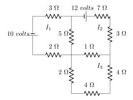
Those jagged places denote resistors and the numbers next to them give their resistance in ohms, written as  $\Omega$ . The breaks in the lines having one short line and one long line denote a voltage source which causes the current to flow in the direction which goes from the longer of the two lines toward the shorter along the unbroken part of the circuit. The current in amps in the four circuits is denoted by  $I_1, I_2, I_3$  and it is understood that the motion is in the counter
