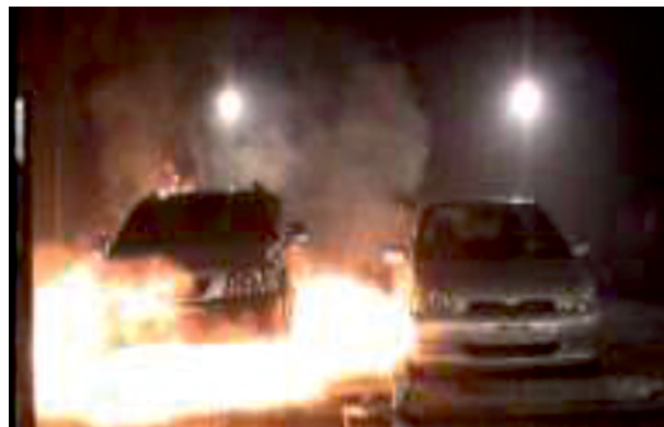
Figure 1–4. The HFCV with initiated TPRD (left) and the gasoline car (right) (Tamura et al., 2011).
