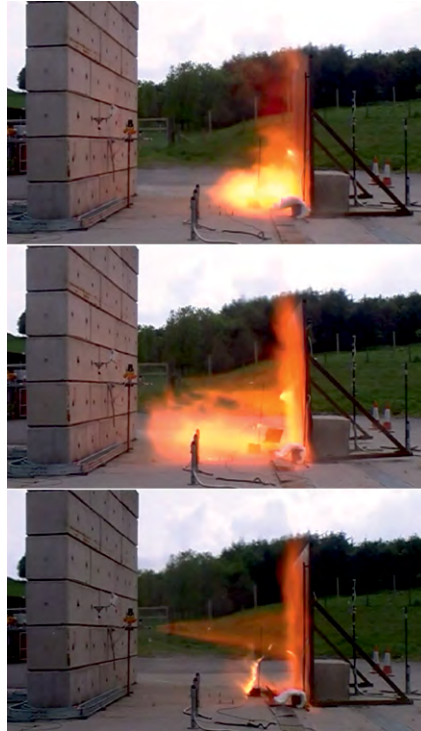
Figure 9-17. The delayed (0.8 s) ignition of hydrogen jet (20.5 MPa pressure storage, 9.5 mm diameter nozzle) impinging a 90 degree barrier: deflagration stage (top and middle snapshot), steady-state impinging jet fire stage (bottom snapshot), HSL test (HYPER, 2008).
