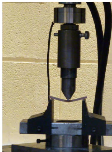
Figure 6.14 A specimen tested in 3-point bending
