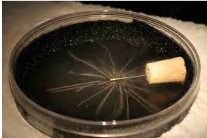
Figure 4.4 Shows tracks consisting of condensed water droplets along the trails of ionization from \alpha particles in a cloud chamber. The end of the needle is a radioactive \alpha particle source (photograph from the Thomas Jefferson National Accelerator Facility – Office of Science Education; available at http://education.jlab.org/glossary/cloud-chamber.html ).
