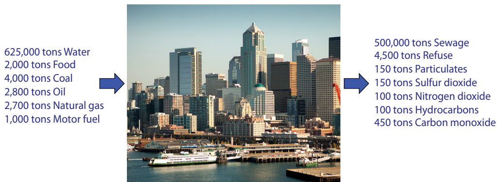
Figure 1.2 The daily metabolism of a city of 1,000,000 people (Wolman 1965). Not all inputs and outputs are listed. (Photo credit: pixabay)
