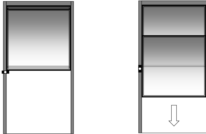
Figure 2.2: Closing a vertical window – irreversibly
